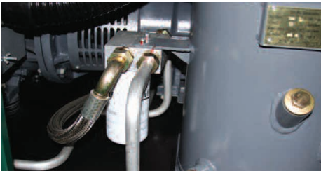
Lubricant filter assembly features a spin-on, full-flow, 12µ, high-efficiency components
